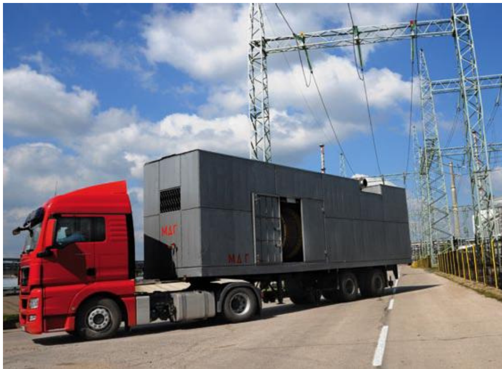
Figure 6.1-3: Kozloduy NPP. Mobile diesel generator.
