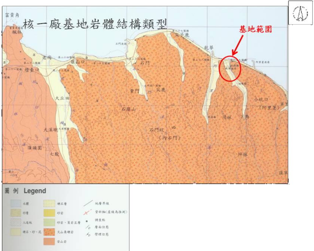
Fig. 4-2 (Lithologic structure type of Chin Shan Power Plant base)
