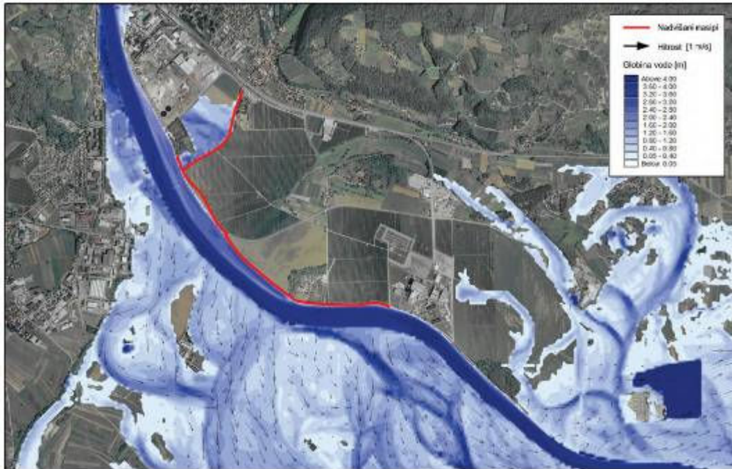
Figure 7: After the completion of modification (increasing the dikes upstream of the plant), the flood at the PMF flow of 7,081 m 3 /s
