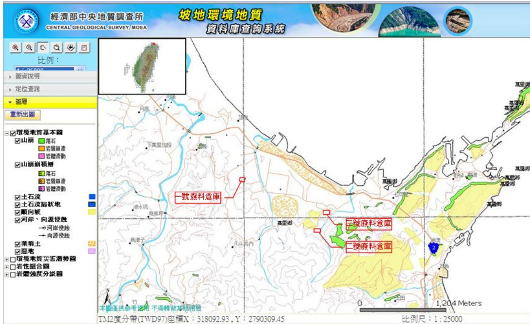
Fig. 4-2 Map of landside susceptible and/or potential debris flow areas near and surrounding Kuosheng site
