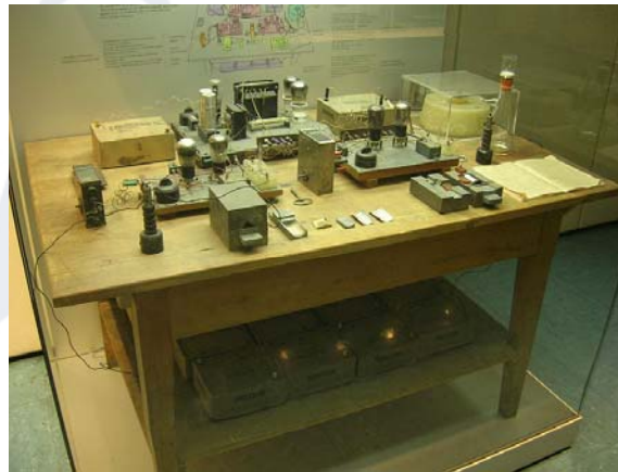
The experimental apparatus with which Otto Hahn and Fritz Strassmann discovered nuclear fission in 1938 © Wikipedia
